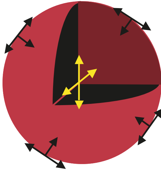
Figure 4.1 Spherical drop of blood in cross-section showing the forces of surface tension.
