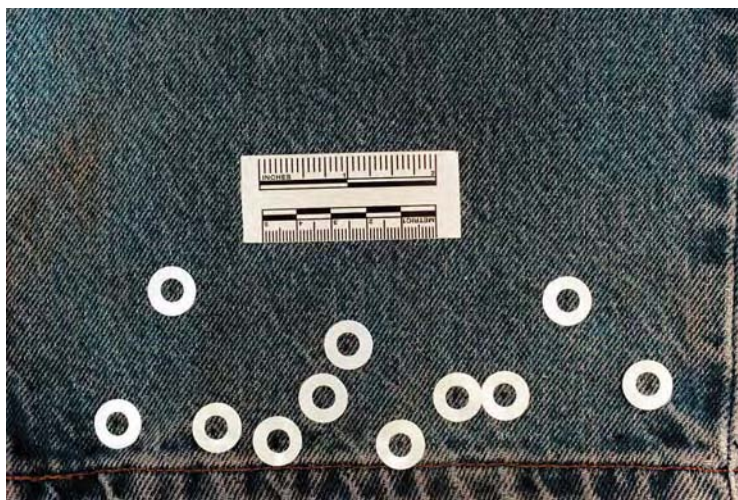
Figure 12.27 Illustrates the use of white self-adhesive ring reinforcers used to visualize the distribution of spatters on denim.
