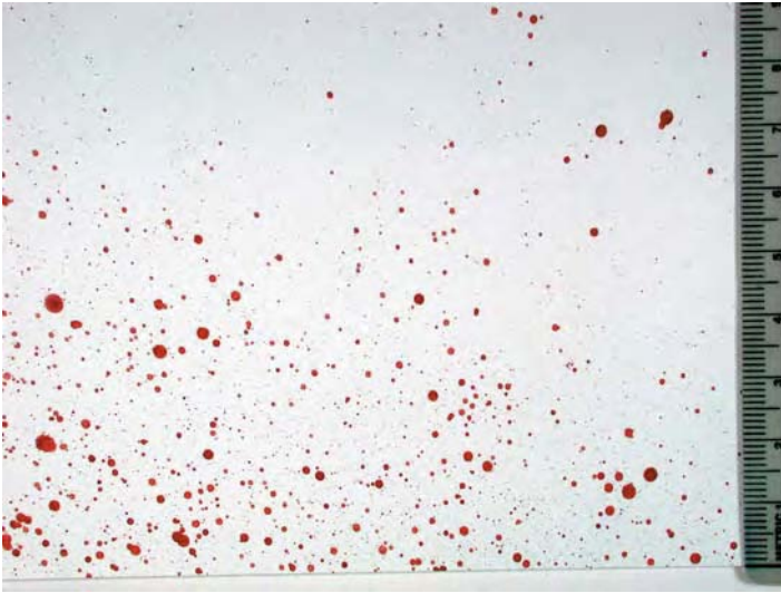
Figure 6.18 Satellite spatters captured on a vertical cardboard target that was positioned next to the impact site of passive drops falling into one another. Zero on the scale represents the same plane as where the blood drops were impacting.
