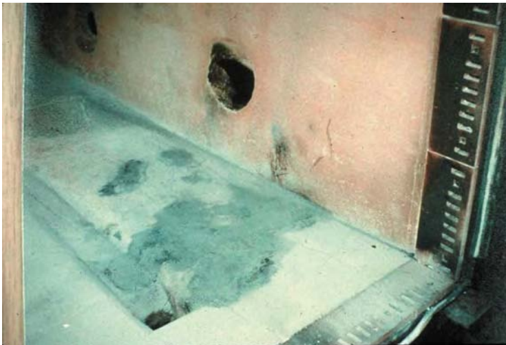
Figure 9.35 Pattern of residue on floor of furnace indicating prior location of victim.
