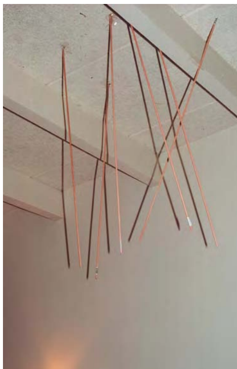
Figure 7.35 View of high-vaulted ceiling with wooden dowels indicating pellet paths and distribution.
