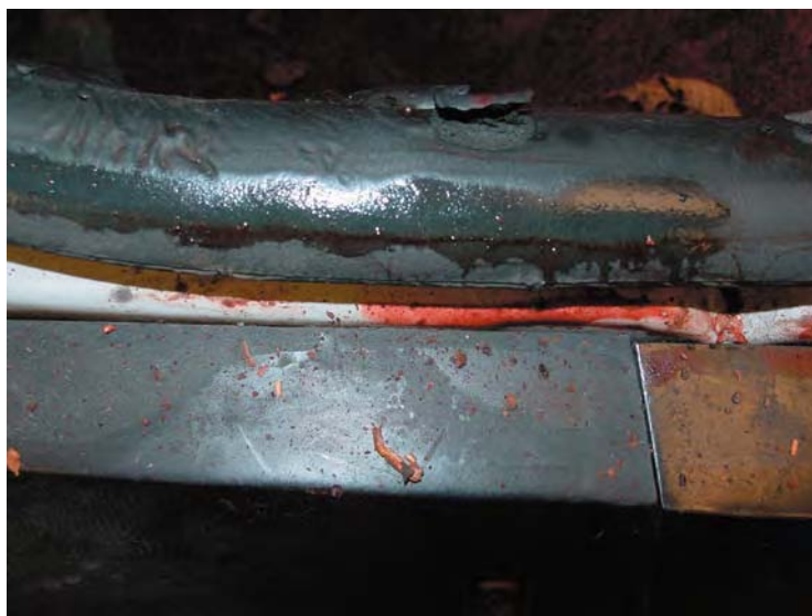
Figure 13.36 Transfer stains on lip of trunk and between the two raised portions of the trunk gasket.
