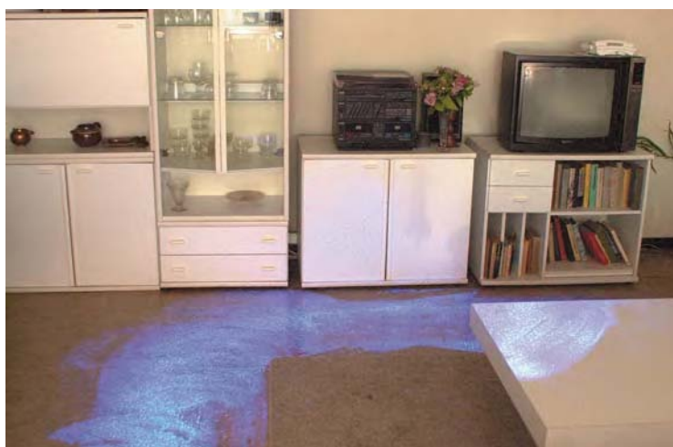
Figure 14.12 Enhancement of area of room subjected to prior cleanup of blood with luminol reagent photographed with digital camera with flash after 27 sec. (Courtesy of Martin Eversdijk, Politie LSOP Institute for Criminal Investigation and Crime Science, Zutphen, The Netherlands.)
