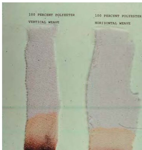
Figure 9.11 Diffusion of blood on 100% polyester cloth with vertical weave strip on left and horizontal weave strip on right.
