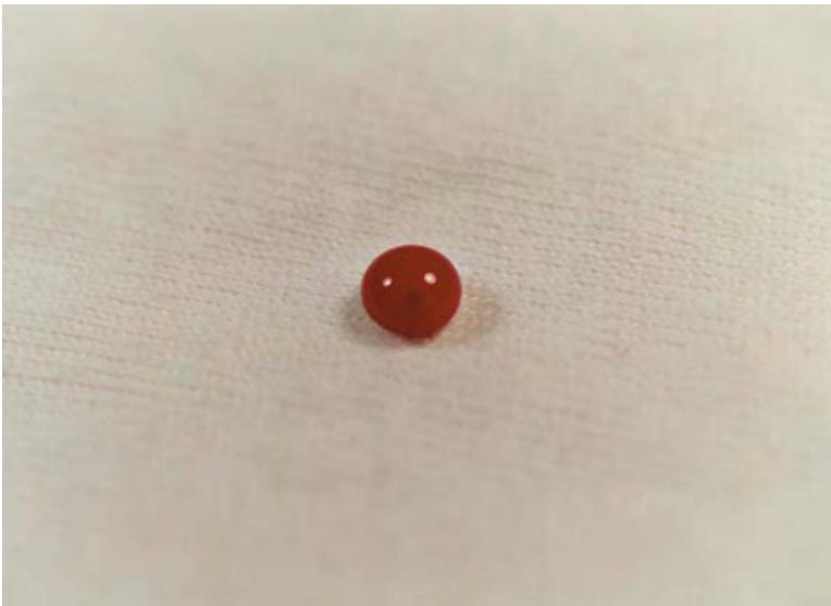
Figure 3.9 Blood drop carefully placed on cotton cloth maintains its shape as a result of cohesion and surface tension.
