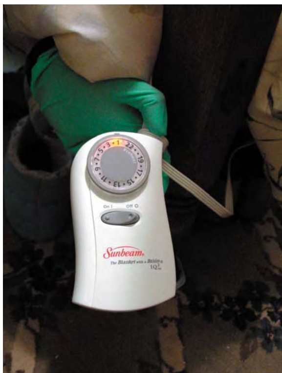
Figure 12.16 Documentation of a bed warmer control. The photograph depicts the exact location of the heat setting and the illuminated indicator light.
