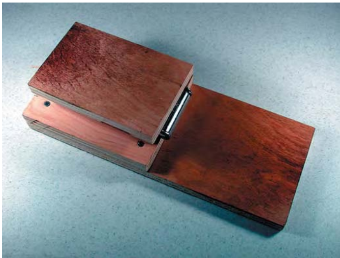
Figure 7.2 Impact spatter apparatus designed to create a reproducible impact to known quantities of blood. A spring-loaded door hinge is used as the source of energy. This causes the upper jaw to be forced down onto the blood located on the base of the apparatus. The amount of energy can be controlled by adjusting the tension on the hinge spring or by releasing the upper jaw from different distances away from the lower base.
