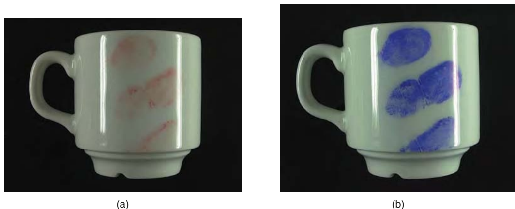
Figure 16.6 (a) A coffee cup with bloody fingerprints prior to enhancement. (b) Coffee cup after treatment with Coomassie Brilliant Blue. Coomassie Brilliant Blue is very suitable for visual enhancement of blood on surfaces made of porcelain or shiny plastics. It will produce a better enhancement result than Amido black methanol-based.
