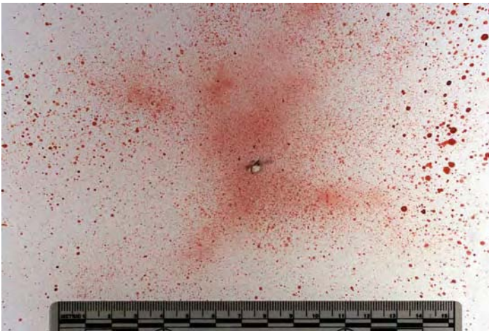
Figure 7.24 Forward spatter produced on vertical cardboard placed 6 in. in front of blood-soaked sponge. Note the true “misting” of the minute stains.
