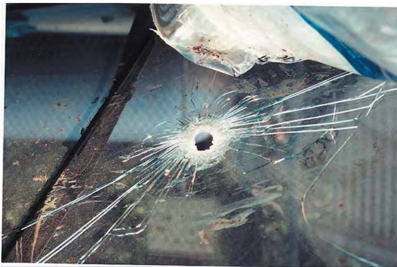
Figure 7.42 Projectile penetration through driver's side windshield of pickup truck. (Courtesy of L. Allyn DeMeo, Arcana Forensics, La Mesa, California.)
