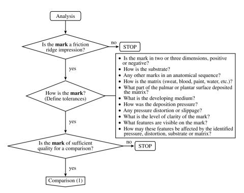
FIGURE 2.3 Flow diagram of the analysis stage.
