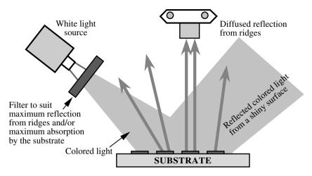
FIGURE 3.28 A schematic representation of the diffused reflection mode.
