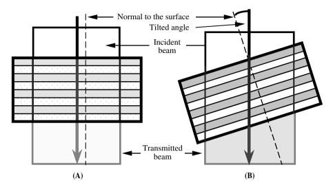
**FIGURE 3.22** (A) Conventional use of an interference filter compared with (B) down-tuning, where the filter is tilted with respect to the incident beam. The light path through the filter layers becomes longer, resulting in a shift of the band toward shorter wavelengths.
