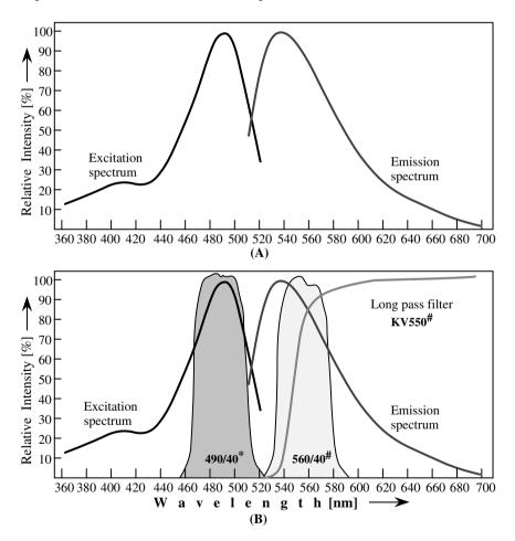
**FIGURE 4.9** (A) Luminescence spectra recorded at liquid nitrogen temperature for a ninhydrin developed print post-treated with zinc nitrate; (B) Recommended filters for excitation (\*) and observation (#) in the luminescence mode.
