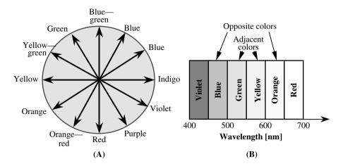
**FIGURE 3.24** The color wheel can be used for the selection of a filter to improve contrast. Colors that are opposite on the wheel are complementary.
