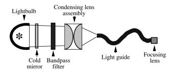
FIGURE 3.39 Schematic representation of a forensic light source.
