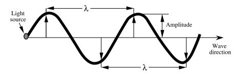
**FIGURE 3.6** Wave theory. Schematic representation of a light wave. The distance between the two nearest points in the same phase is known as the wavelength  $\lambda$ .
