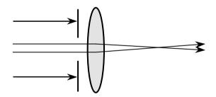
**FIGURE 3.43** A diaphragm in front of the lens reduces the lens aperture, thus reducing the spherical aberration effect.
