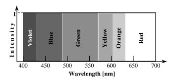
**FIGURE 3.8** When each color (wavelength) of the visible spectrum is present with the same relative intensity, we have white light.
