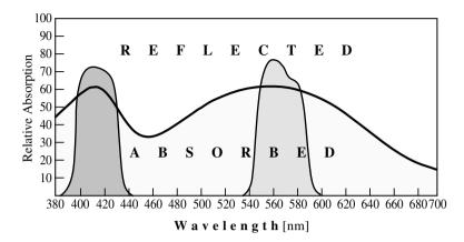
**FIGURE 3.27** A typical absorption spectrum for a ninhydrin-developed fingerprint. There are two absorption bands: a narrow band with a maximum at around 410 nm (violet region) and a broad major band with a maximum at around 560 to 580 nm (green–yellow region).
