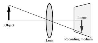
FIGURE 3.41 Formation of an image using a lens.
