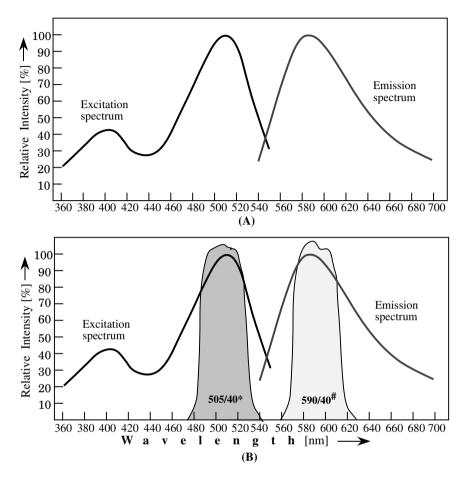
**FIGURE 4.10** (A) Luminescence spectra recorded at liquid nitrogen temperature for a ninhydrin developed print post-treated with cadmium nitrate; (B) Recommended filters for excitation (\*) and observation (#) in the luminescence mode.
