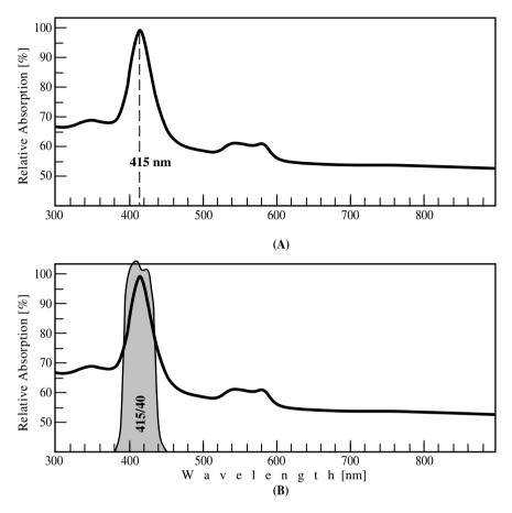
**FIGURE 4.31** (A) Relative absorption spectrum of dry blood, showing a strong absorption peak at 415 nm. (B) Recommended bandpass filter for observation in the absorption mode.
