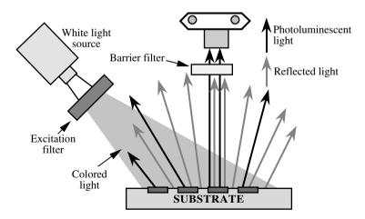
FIGURE 3.34 Arrangement for photoluminescence observation.
