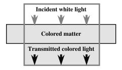
FIGURE 3.20 White light filtered through an energy-absorbing filter.
