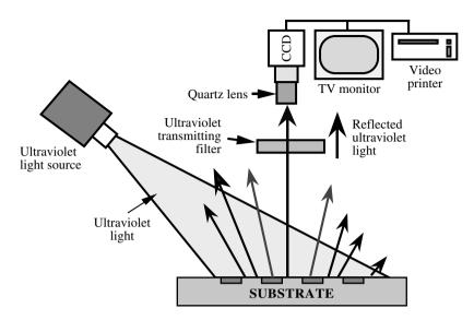
FIGURE 3.38 Implementation of the UV reflection mode.
