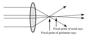
FIGURE 3.42 Schematic representation of spherical aberration.
