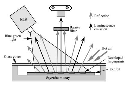
**FIGURE 4.11** General luminescence mode set-up for the recording of ninhydrin developed prints post-treated with a metal salt (zinc or cadmium).
