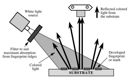
**FIGURE 3.26** Schematic representation of the absorption mode with the appropriate filter in front of a light source. This method can be used only in dark or semidark situations.
