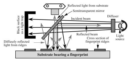
**FIGURE 3.30** A schematic representation of episcopic coaxial illumination. (From Pfister, R. [1985], The optical revelation of latent fingerprints, *Fingerprint Whorld*, 10, 64–70. With permission.)
