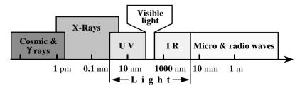
**FIGURE 3.5** The electromagnetic spectrum. Light consists of three parts: ultraviolet (UV), visible, and infrared (IR). Visible light is a very small portion in this region.
