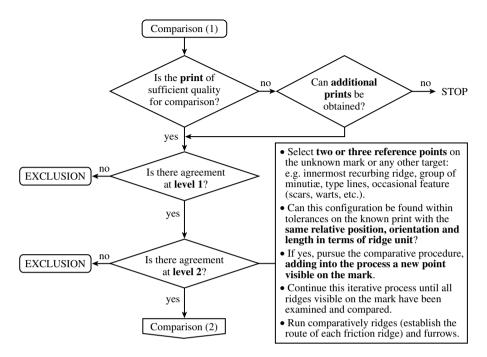
FIGURE 2.4 Flow diagram (part 1) of the comparison stage.
