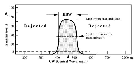
FIGURE 3.18 Typical transmission characteristics of a bandpass filter.
