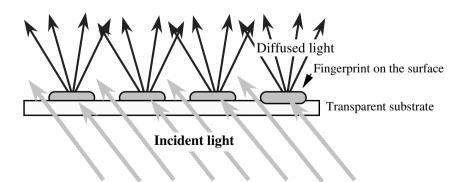
**FIGURE 3.29** The diffused reflection mode as applied to a transparent substrate. Note that the incident light is directed at an angle from underneath the object.
