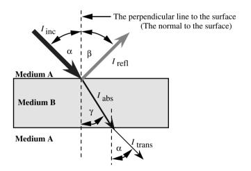
FIGURE 3.12 Transformation of incident light after irradiation of an object.
