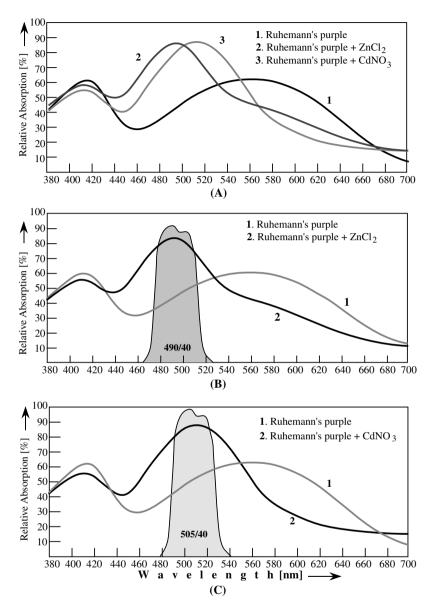
**FIGURE 4.8** (A) Relative absorption spectra of Ruhemann's purple and its complexes with zinc and cadmium; (B) Recommended bandpass filter for observation in the absorption mode in the case of the zinc complex; (C) Recommended bandpass filter for observation in the absorption mode in the case of the cadmium complex.
