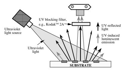
**FIGURE 3.37** Typical setup for the photoluminescence mode with excitation in the UV region and observation in the visible region.
