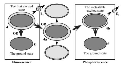
**FIGURE 3.15** The molecule in stage 4 (first excited state) has two possibilities of returning to the ground state: directly, or indirectly by further sharing its extra energy. The latter process takes longer and leads to phosphorescence emission.
