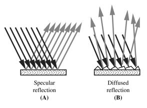
FIGURE 3.13 (A) Specular reflection from a flat surface. (B) Diffused reflection from a rough surface.
