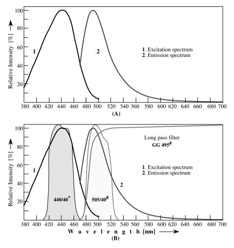
**FIGURE 4.23** (A) Luminescence spectra for a cyanoacrylate-developed fingerprint stained with Basic Yellow 40; (B) Recommended filter combination for excitation (\*) and observation (#).
