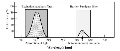
**FIGURE 3.32** Absorption and emission curves for a theoretical photoluminescent material with choice of appropriate excitation and barrier filters.
