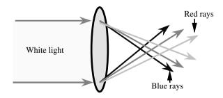
FIGURE 3.44 Schematic representation of chromatic aberration.
