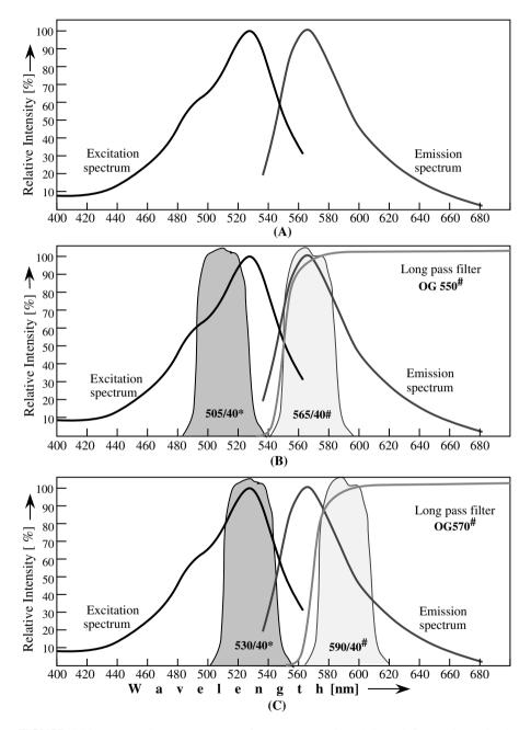
**FIGURE 4.22** (A) Luminescence spectra for a cyanoacrylate-delivered fingerprint stained with rhodamine 6G; (B, C) recommended filter combinations for excitation (\*) and observation (#) mode.
