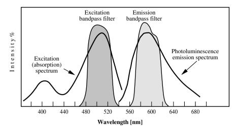
**FIGURE 3.33** Excitation and emission spectra for a ninhydrin-developed latent fingerprint post-treated with cadmium nitrate (as an example) with the choice of appropriate filters for excitation and emission.
